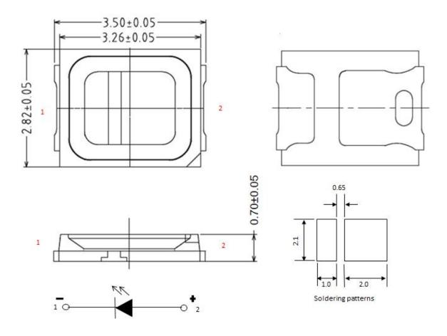
NOTE: All dimensions in mm tolerance is ±0.1mm unless otherwise noted.
