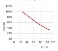
Fig.5 Maximum Forward Current VS. Ambient Temperture
