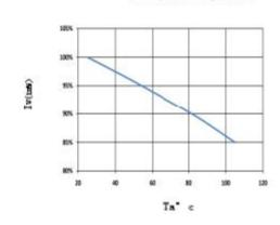
Fig.4 Relative Luminous Intensity
