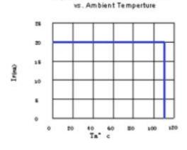
Fig.5 Maximum Forward Current
