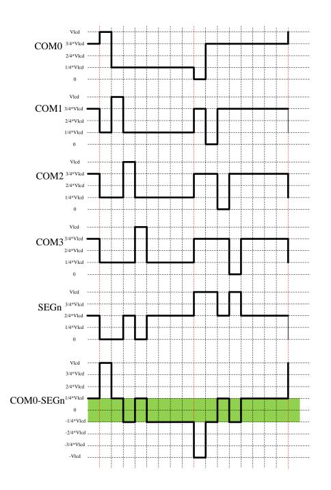
LCD timing diagram (1/8 duty cycle, 1/4 bias)
