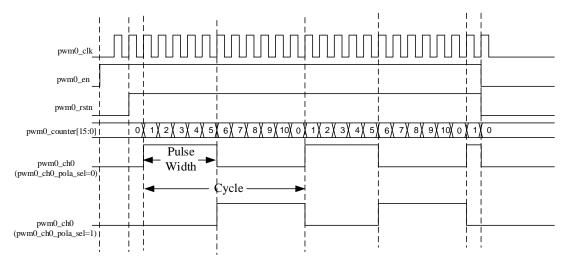
PWM0 output waveform (PWM0\_DUTY\_CH0=5, PWM0\_MOD=10, duty\_cycle=5/11)
