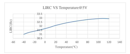
$f_{\mbox{\sc LIRC}}$  temperature curve
