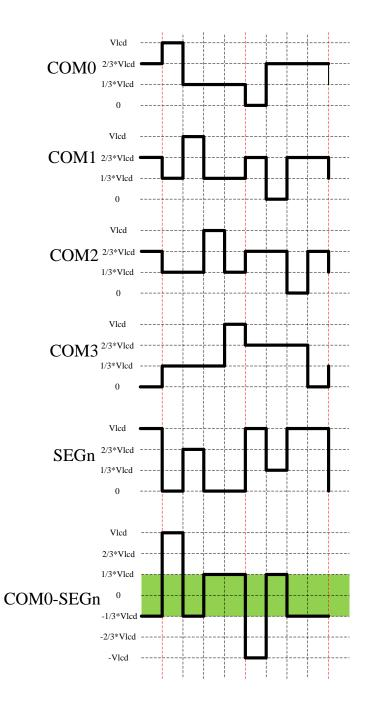
LCD timing diagram (1/4 duty cycle, 1/3 bias)
