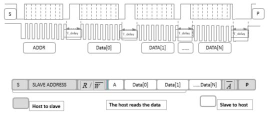
PS: T\_delay: Reserve slave interrupt time, generally 60us^300us, if the slave IIC interrupts the service processing time at100us, suggest T\_delay>200us.
