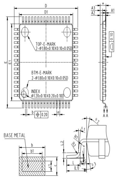
COMMON DIMENSIONS (UNITS OF MEASURE=MILLIMETER)
