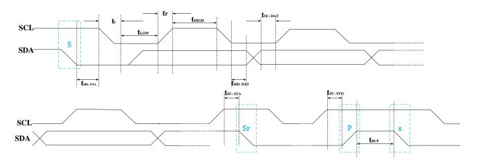
S: Start signal, SCL and SDA lines are high at the same time, and a signal from high to low appears on the SDA line.
