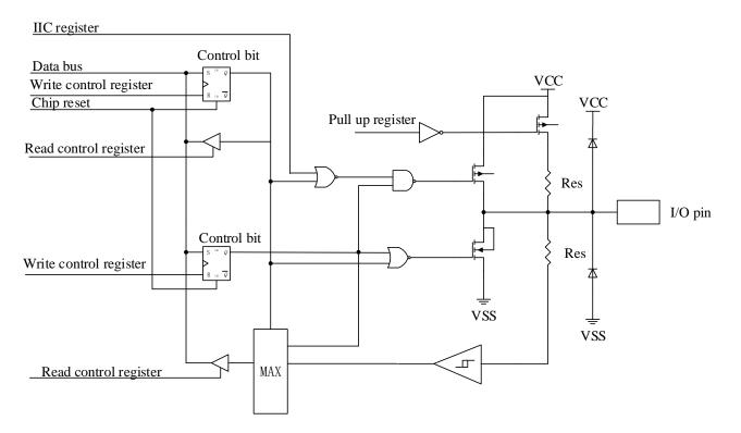
Open drain output IO structure diagram
